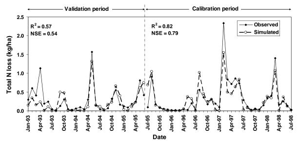
Figure 20. Observed and simulated Total N loss for the calibration and the validation periods at the Hico monitoring station
