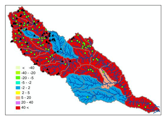
Figure 49d. % Change Total P Flow Accumulation No Reservoirs All Manure Applied
