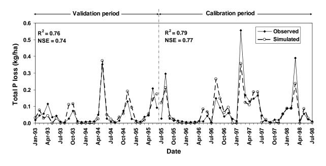
Figure 21. Observed and simulated Total P loss for the calibration and the validation periods at the Hico monitoring station
