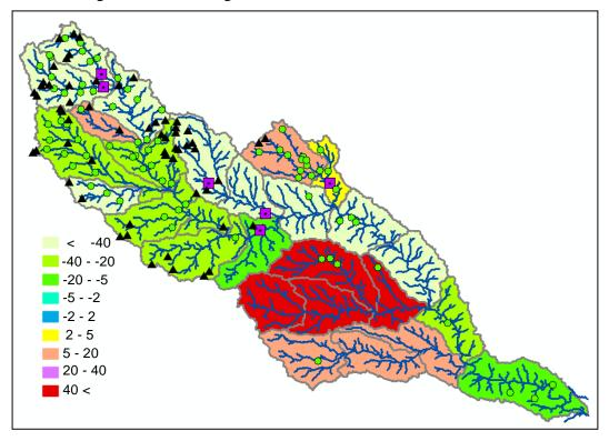
Figure 55d. % Change Total P Flow Accumulation ICIPG-Added Reservoirs-Hauloff
