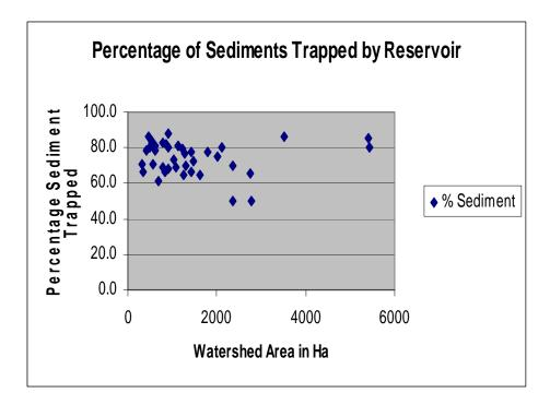
Figure 63. Sediment Trapped in NRCS Reservoirs
