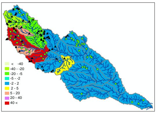
Figure 45h. % Change Mineral P in Water DWMA-Existing Reservoirs All Manure-Applied
