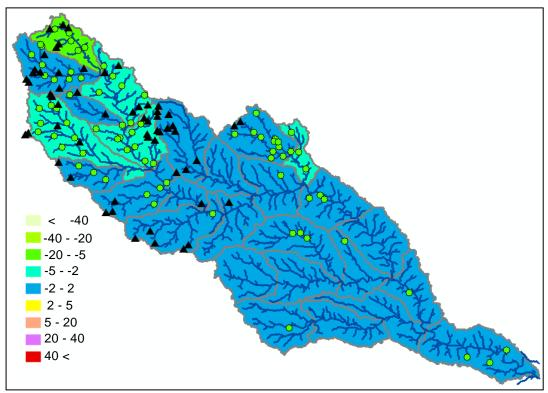
Figure 49h. % Change Mineral P in Water No Reservoirs All Manure Applied
