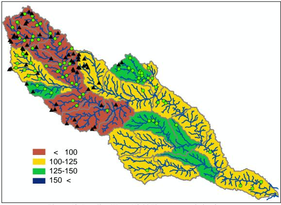
Figure 42. Baseline Water Yield Flow Accumulation in mm
