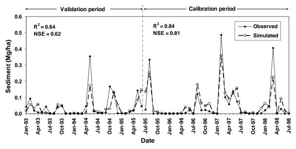
Figure 19. Observed and simulated sediment yield for the calibration and the validation periods at the Hico monitoring station
