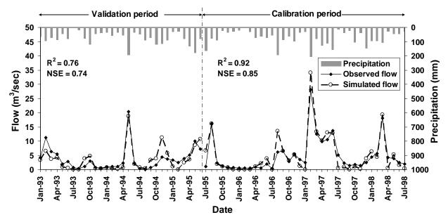
Figure 18. Observed and simulated flow for the calibration and the validation periods at the Hico monitoring station
