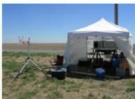
Figure 1. Disjunct eddy accumulation system for measuring N 2 O flux and the UV differential optical absorption spectroscopy for NH 3 and NO measurements.
